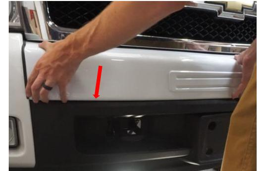
5. Ensure that the bumper cover is properly positioned. (There should be no, or very little bumper surface visible at this point). Re-adjust, as necessary.
