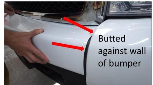
4. Align the front, vertical surface, such that the lower flange tucks into the seam between the bumper and the lower trim, being careful to minimize contact of the tape with the bumper.
