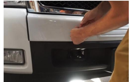
7. Finally, put firm pressure and the taped areas on the top of the bumper cover, near the grill, to finish the attachment process. The tape spans the entire width of the cover below, and slightly forward of the grill.
