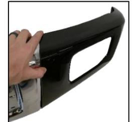
6. Install center cover by first removing red backing of 3M tape. Apply center cover over center bumper section, with the edges overlapping the side covers. If you were not able to remove the top trim, use a plastic trim tool or credit card to pry up on the trim enough to slip the top edge of the cover all the way underneath. Try not to allow taped areas to touch until BumperShell is located correctly.
