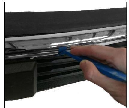
2. Removing the bumperettes will allow easy access to the clips that secure the upper trim piece on top of the front bumper on some F150 models. If these clips are not accessible, removal is NOT necessary for the final install, but may make installation a little easier.
