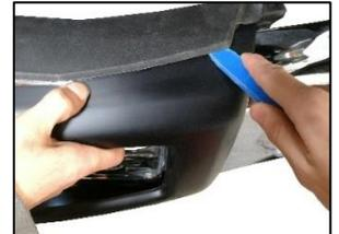
7. Finally, begin putting firm pressure on all areas of the BumperShellz where the 3M tape will be contacting the bumper. Be thorough to ensure best adhesion.
