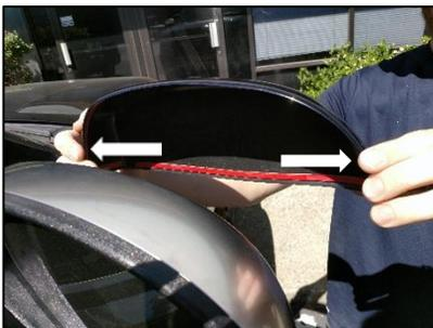
6. Tip the top edge of the mirror cover towards yourself, so only the bottom edge of the cover will come into contact with the factory mirror cap.
