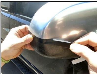
4. Remove red backing to 3M double-sided tape on reverse side of Mirror Cover
