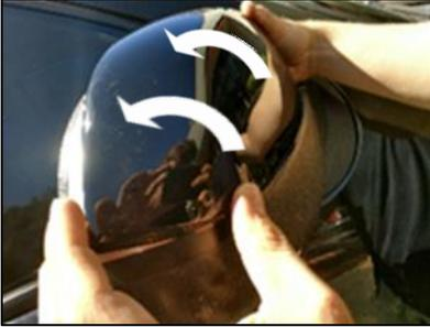
8. Check around each side of the cover to ensure that no chrome is visible before you begin putting pressure on the taped areas. Shift the cover if necessary to perfect the fitment. After you are satisfied with the fitment of the cover, begin putting pressure on all taped areas.
