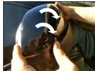
7. Slowly tip the top edge of the cover back towards the mirror making sure that the bottom edge of the MirrorShell continues to cover all the original factory mirror cap.
