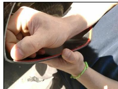
5. Begin installing the mirror cover by carefully pulling the edges out to widen the opening which will decrease the likelihood of the tape touching down prematurely.
